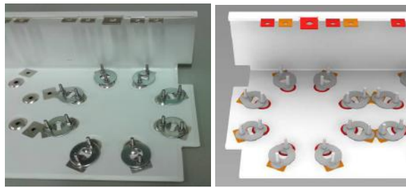
Fig. 15: Actual bus bar setup and 3D model for measurement and simulation, respectively.
