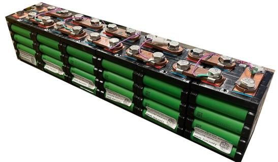
Fig. 7. One of the six segments used to create the battery.
