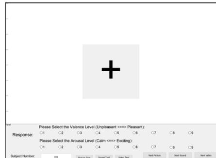
Figure 21: GUI of the application used to collect data for training and evaluating our real emotion classifier. Users are shown a stimulus through the GUI and are asked to select their arousal and valence level after each stimulus.
