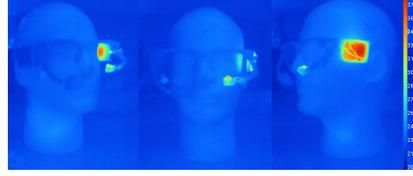
Figure 4: Thermal image of SPIDERS+ in the active mode.
