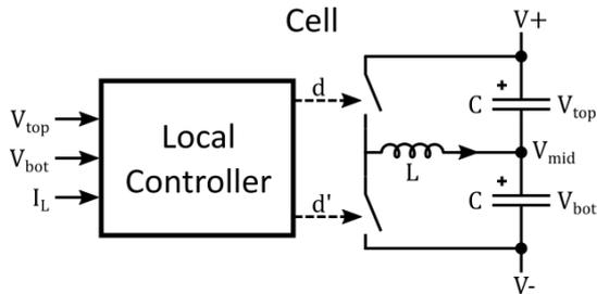
Fig. 2: Single cell with local feedback
