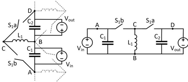
Fig. 3: Stackable unit cell as it relates to the inverting buck-boost converter (dashed lines show connections of adjacent cells).
