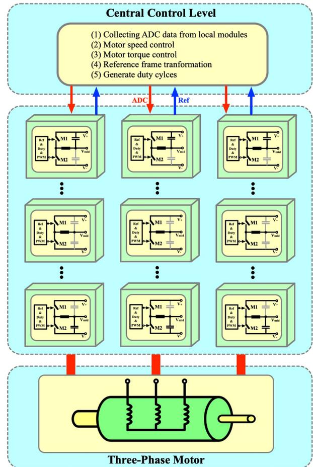
Fig. 1: Software-defined stacked control architecture for motor application
