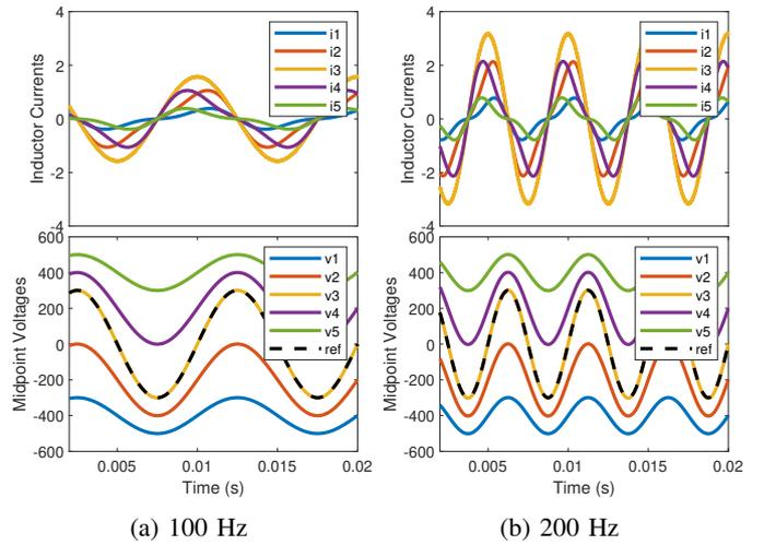
Fig. 6: Circulating currents increase with frequency.
