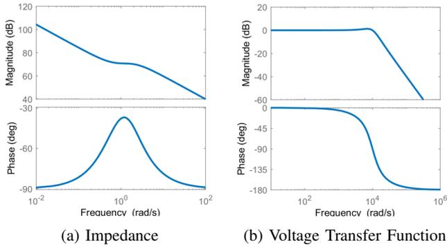
Fig. 11: Cell approximate impedance and transfer function.
