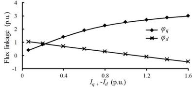
Fig. 3 Flux linkage at different load conditions.  $\phi_d(-I_d)$  and  $\phi_q(I_q)$ .
