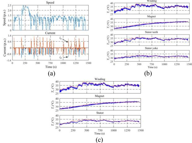
Fig. 7 Experimental validation on UDDS drive cycle. (a) UDDS procedure. (b) Estimation by 4-node model. (c) Estimation by 3-node model. (Figure b and c, red lines: estimates, blue lines: measurement).
