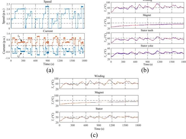
Fig. 6 Experimental validation on heavy load test. (a) Heavy load procedure. (b) Estimation by 4-node model. (c) Estimation by 3-node model. (Figure b and c, red lines: estimates, blue lines: measurement).
