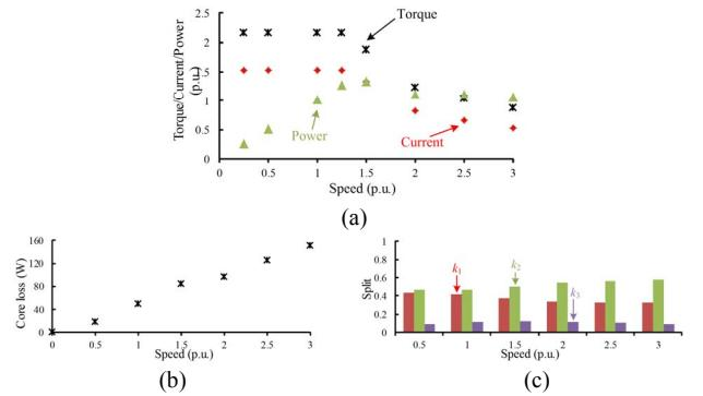
Fig. 1 FEA loss calculation. (a) Operation conditions for calculation. (b) Core Loss. (c) Split coefficients.
