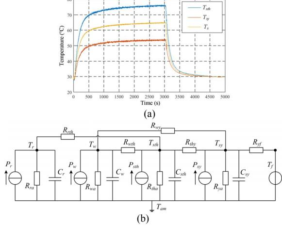
Fig. 2 Building the thermal network. (a) Temperature curves on stator teeth and yoke, and their average, operation condition: 1 per unit torque and 1 per unit speed. (b) 4-node thermal network for IPM motor.
