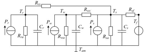
Fig. 4 Reduced 3-node thermal network.
