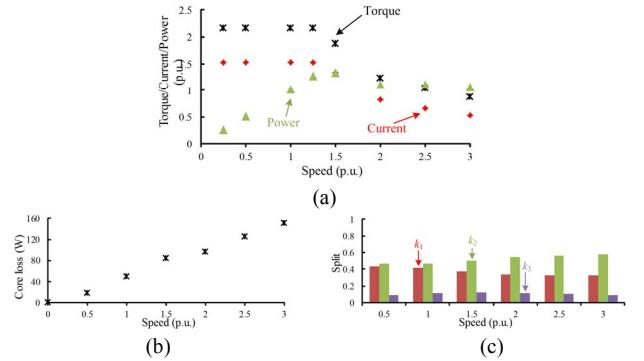
Fig. 1 FEA loss calculation. (a) Operation conditions for calculation. (b) Core Loss. (c) Split coefficients.
