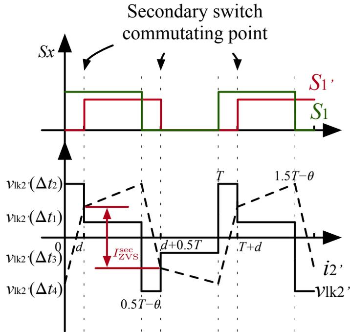
Figure 5.2: The worst primary leakage ripple current with different coupling factors and effective turns ratios
