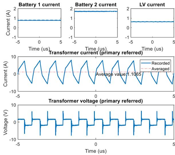
Figure 3.43: Experimental validation of Mode A C2LV + C2C with unequal cell currents
