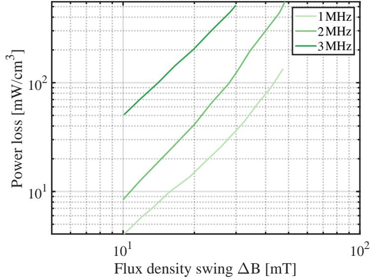
Figure 3.28: The core loss density vs. flux density swing at 1, 2, and 3 MHz switching frequency
