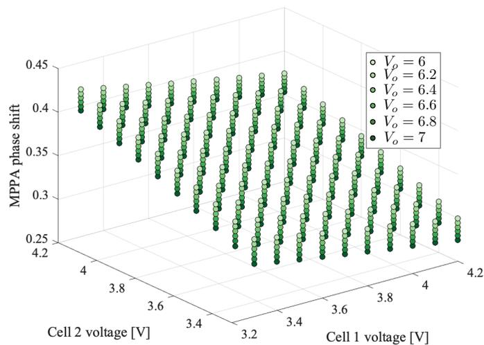
Figure 5.10: The MPPA phase shift with different combinations of cell voltages
