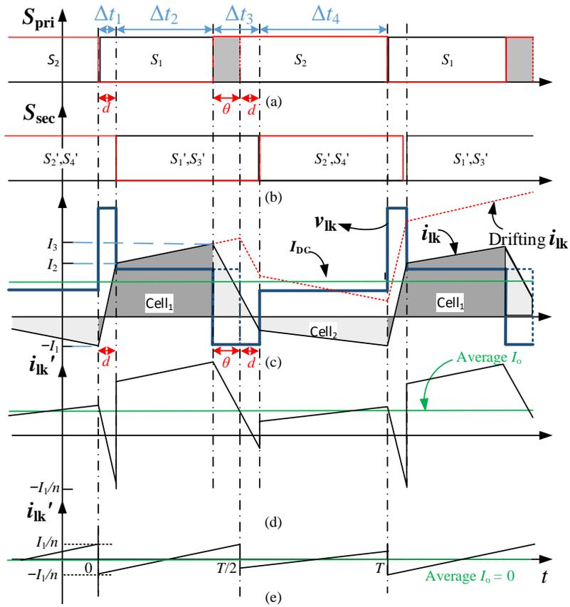
Figure 3.5: Switching PWM signals: (a) primary switches, (b) secondary switches; (c) primary referred leakage inductor voltage and current: red dot - symmetric control, black line - asymmetric control; secondary-referred leakage inductor current (d) with phase shift and (e) without phase shift
