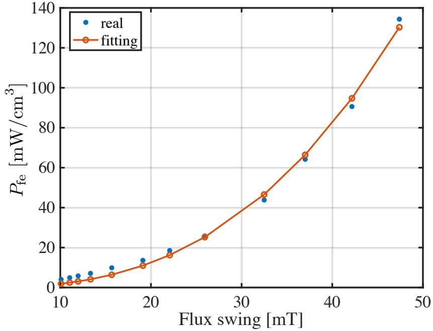
Figure 3.29: Core loss curve fitted at 1 MHz
