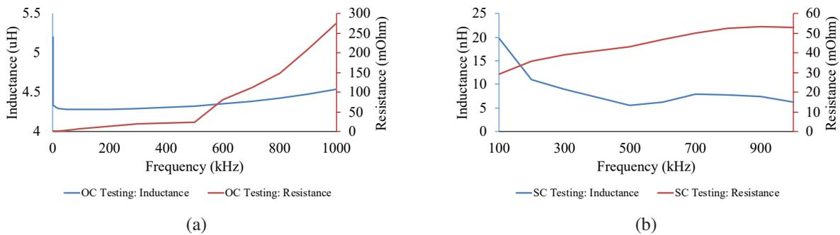
Figure 3.35: Measurements of inductance and resistance (a) OC measurements, (b) SC measurements
