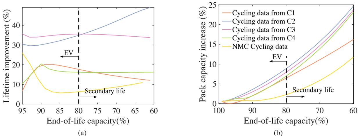
Figure 2.9: The benefits of redistributive balancing in (a) life extension within 40% weakest cell capacity loss, (b) increase of pack capacity utilization within 40% weakest cell capacity loss. C1: [29], C2: [30], C3: [31], and C4: [32]
