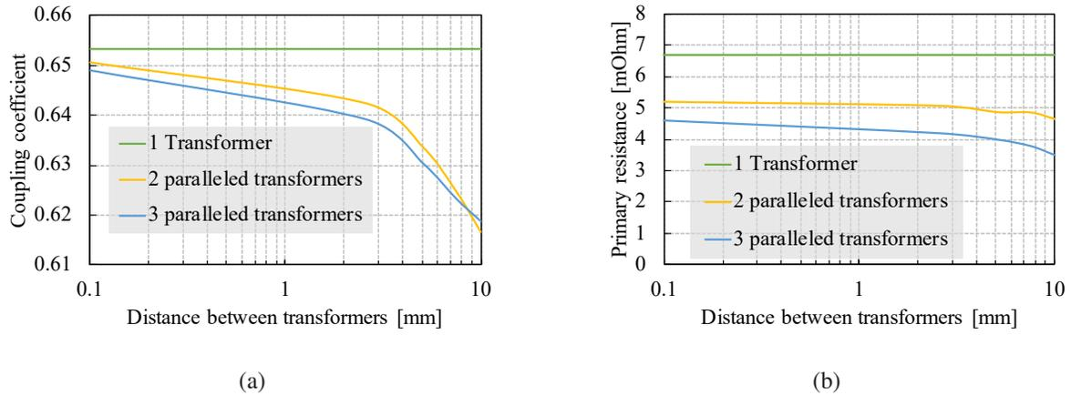
Figure 4.22: The simulated effect of distance between paralleled transformers on (a) coupling coefficient and (b) primary resistance, with a winding inner radius of 20 mm
