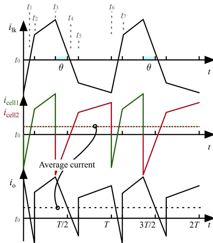
Figure 3.9: The current waveforms when battery are unbalanced, top: leakage inductor current on primary side; middle: cell currents; bottom: output current on LV side
