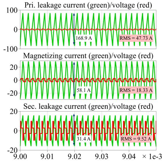
Figure 4.14: Model vs. simulation at worst case when  $a = 3.5$
