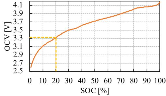
Figure 3.17: The OCV-SOC curve of the NMC cell
