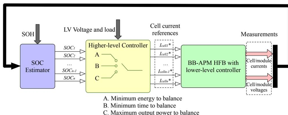
Figure 3.36: Higher-level controller distributing power demands to each local controller
