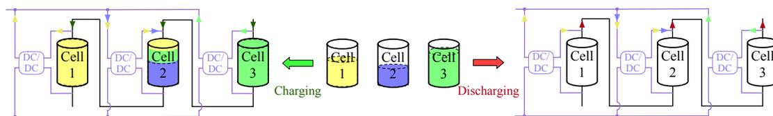
Figure 2.5: The balancing results utilizing redistributive balancing strategy
