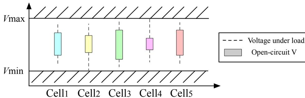
Figure 2.6: Early triggered protection due to the impedance mismatch
