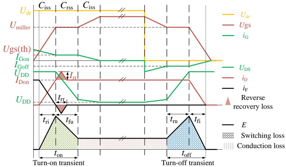
Figure 5.9: The switching transient of a MOSFET
