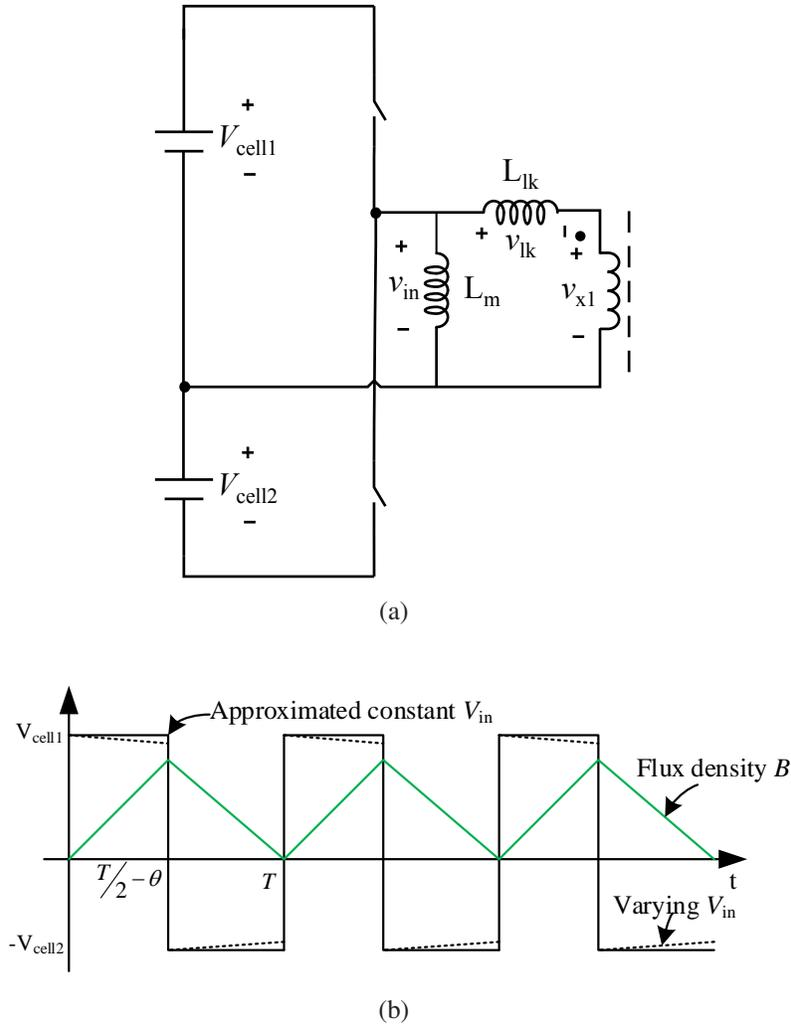
Figure 3.21: (a) Primary-side simplified circuit, (b) Flux density due to applied voltage
