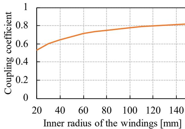
Figure 4.20: The coupling coefficient vs. windings inner radius
