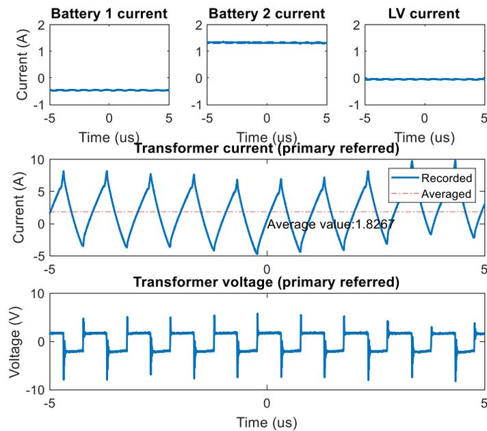
Figure 3.46: Experimental validation of Mode D C2C only
