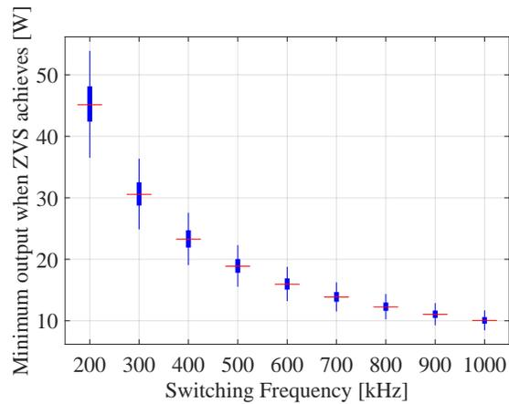
Figure 5.5: The minimum output power when soft switching is enabled at different frequencies
