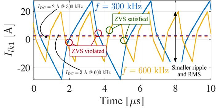
Figure 5.4: The measured waveforms of leakage inductor current at 300 kHz and 600 kHz
