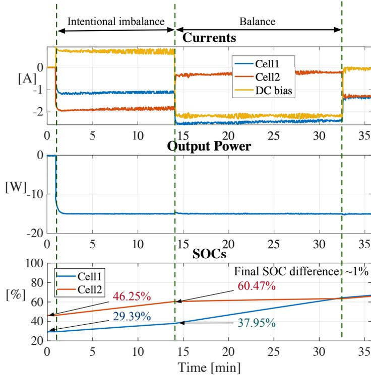
Figure 3.49: Experimental balancing functionality tests on two 3000 mAh NMC cells with intentional imbalance and balance for charging
