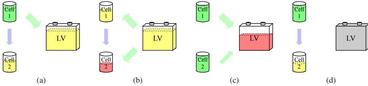
Figure 3.12: The feasible balancing modes: (a) C2C and C2LV, (b) C2C and LV2C, (c) C2LV only, and (d) C2C only
