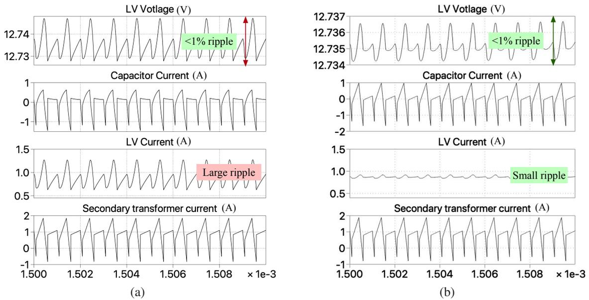
Figure 3.15: Simulation results of output current ripple with 4.2 V and 2.7 V cell voltages: (a) 10  $\mu\text{F}$  filtering capacitance, (b) 66  $\mu\text{F}$  filtering capacitance
