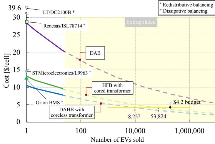
Figure 6.8: The cost difference among the HFB with core, coreless DAHB and the DAB configurations
