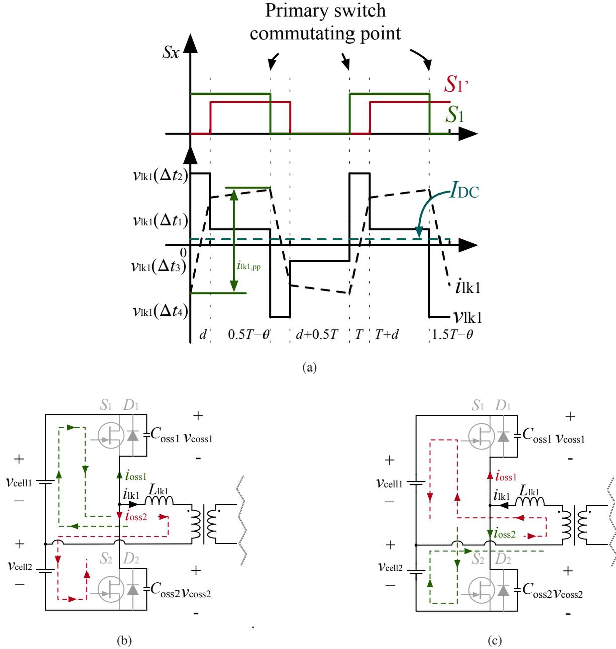
Figure 5.1: The ZVS condition for primary switches: (a) the primary leakage inductor current waveform; the current flow to achieve ZVS: (b) at time instance of  $0.5T - \theta$ , (c) at time instance of  $T$
