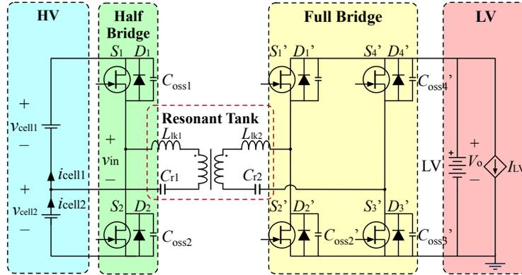
Figure 4.3: The potentially feasible CLLC converter, modified based on proposed HFB converter
