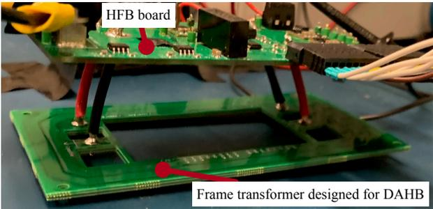
Figure B.1: The HFB with the frame coreless transformer on
