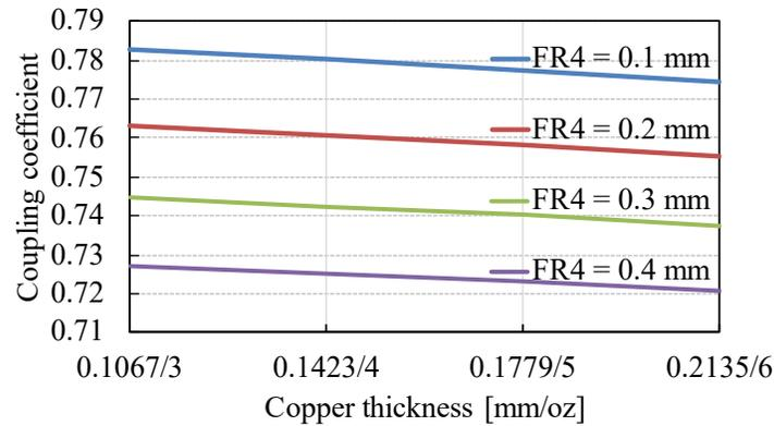
Figure 4.21: The coupling coefficient vs. copper and FR4 thickness
