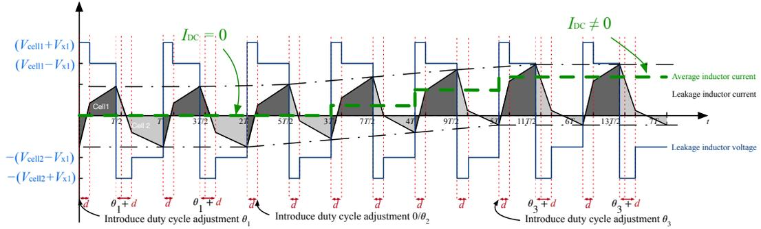
Figure 3.11: The process of regulating  $I_{DC}$  to introduce a non-zero  $I_{DC}$
