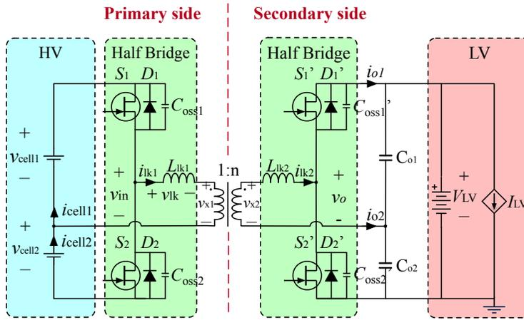
Figure 4.4: DAHB topology with coreless transformer
