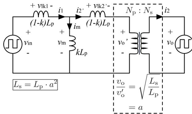
Figure 4.6: The equivalent transformer model considering the coupling factor and nonideality
