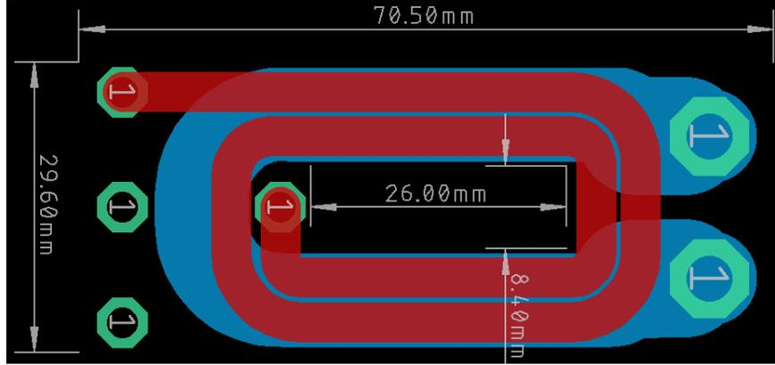
Figure 3.25: The dimensions for calculating the *MLT* for the designed transformer
