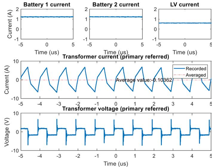
Figure 3.45: Experimental validation of Mode C C2LV only with equal cell currents
