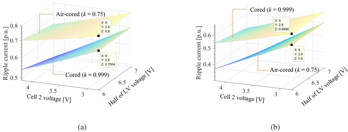
Figure 4.11: Per-unit (a) primary leakage secondary inductor ripple current with the same leakage inductance, (b) primary-referred leakage inductor ripple current with the same leakage inductance
