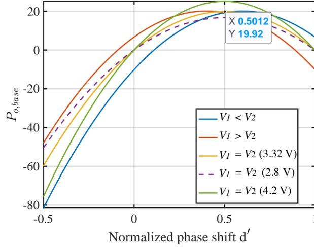
Figure 4.17: Output power in p.u. system at extreme conditions
