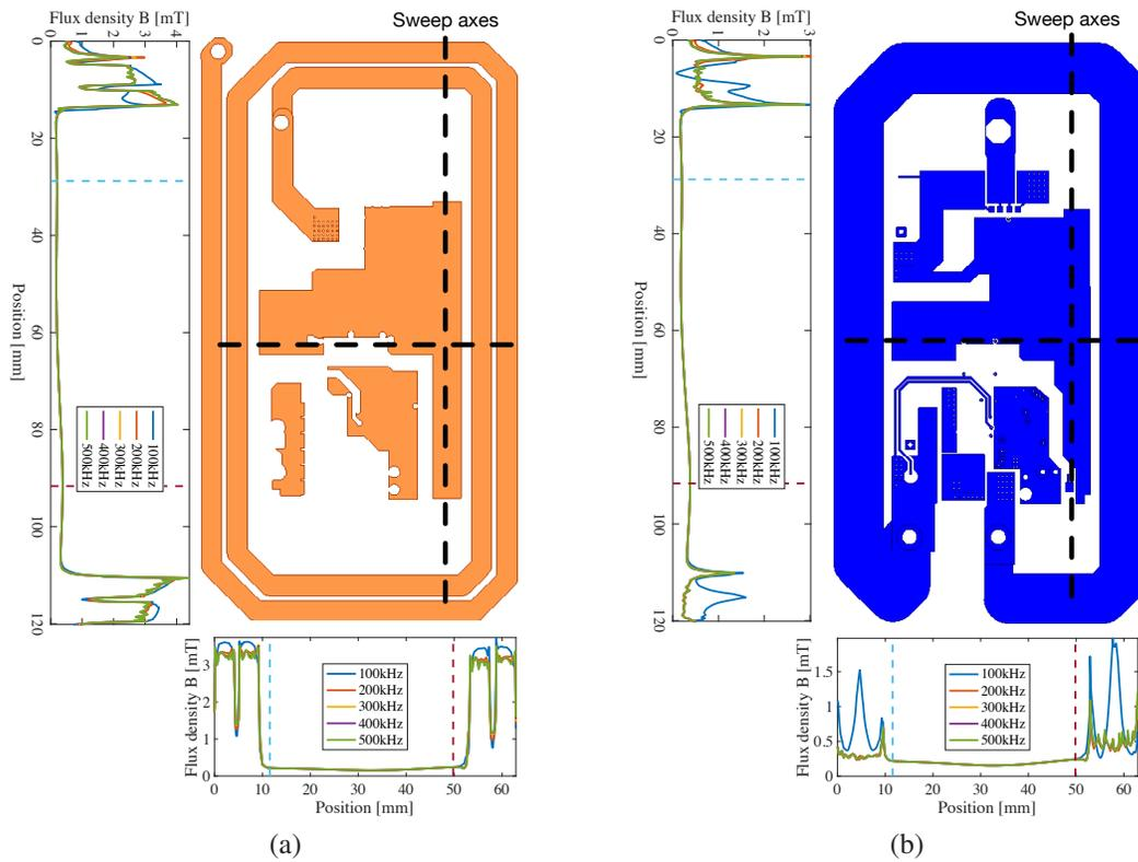
Figure A.2: The flux density distribution on (a) the layer-3 and (b) bottom PCBs
