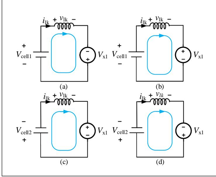
Figure 3.6: Equivalent circuit models referred to primary side during: (a)  $0 \leq t < d$ , (b)  $d \leq t < \frac{T}{2}$ , (c)  $\frac{T}{2} - \theta \leq t < \frac{T}{2} + d$ , and (d)  $\frac{T}{2} + d \leq t < T$
