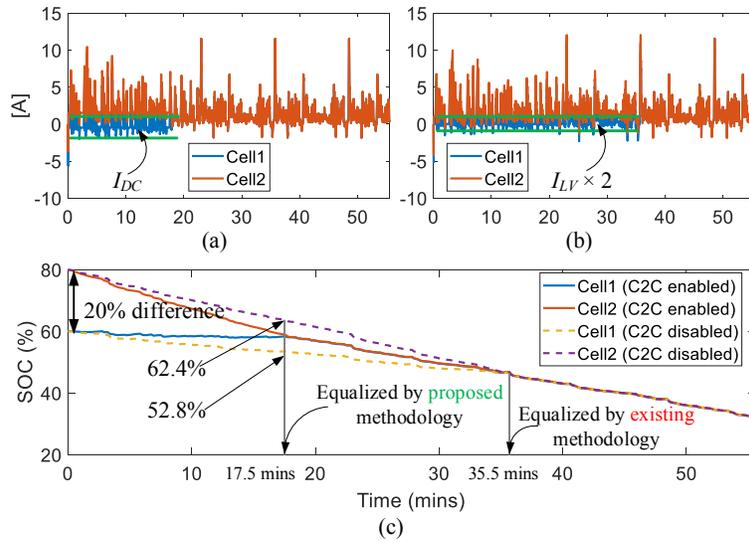
Figure 3.53: Simulation results leveraging non-C2C APM and proposed methodology with combination of UDDS and US06 driving cycles: (a) cell currents with C2C enabled, (b) cell currents without C2C, (c) comparison of balancing performance in terms of SOC
