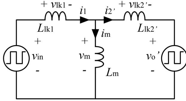
Figure 4.5: The equivalent circuit model of the transformer with the square-wave input voltage sources
