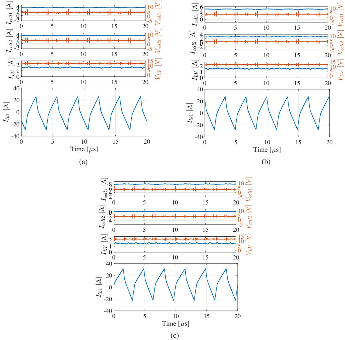
Figure 4.27: The measured waveforms at 300 kHz when consuming 30 W with (a)  $I_{DC} = 0$  A, (b)  $I_{DC} = 2$  A, (c)  $I_{cell2} = 0$  A, cell 1 providing full power (replotted in MATLAB)
