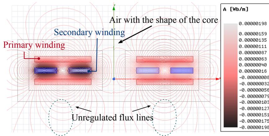
Figure 4.2: Distribution of flux lines for a transformer without core
