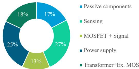
Figure 6.7: The HFB cost breakdown for optimized batch production for HFB
