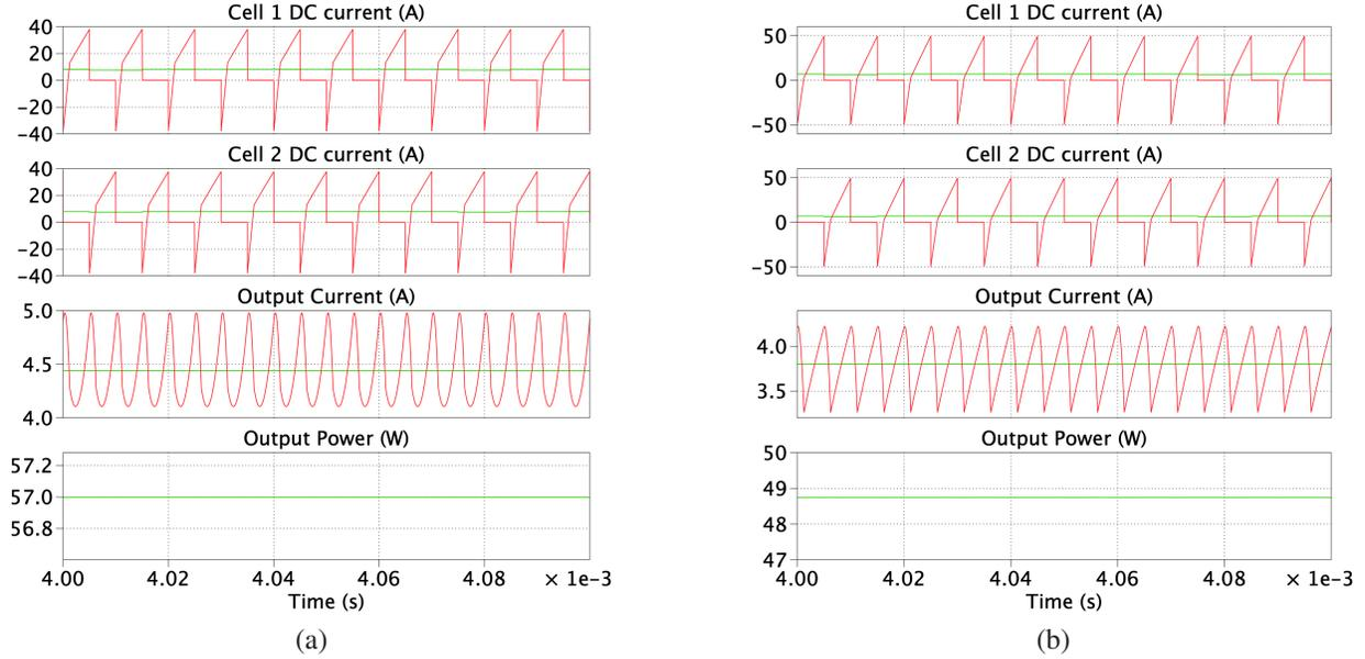
Figure 4.16: The output power simulation with (a)  $k = 0.999$  and (b)  $k = 0.75$
