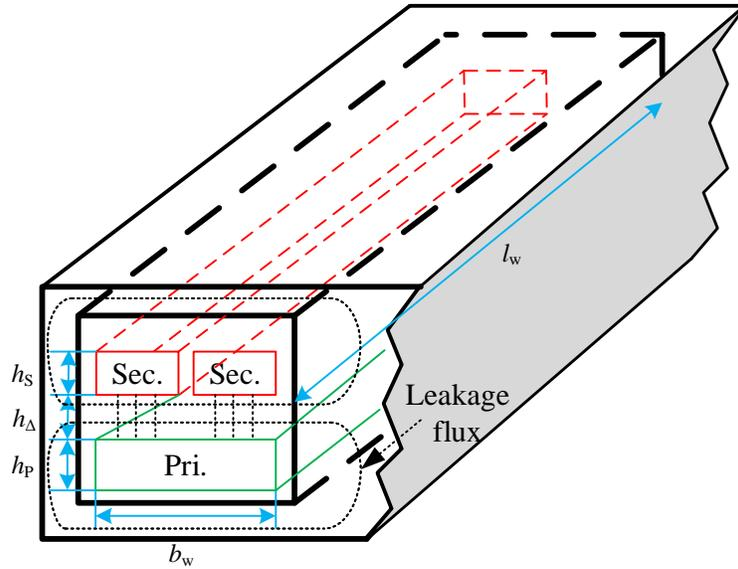
Figure 3.22: The diagram of flux leakage in a simplified 1:2 transformer
