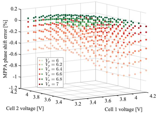
Figure 5.13: The MPPA phase shift error between 4th-order model and full-order one
