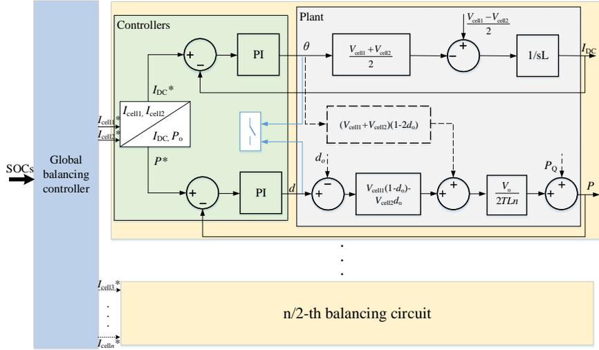
Figure 3.37: Diagram of lower-level controller
