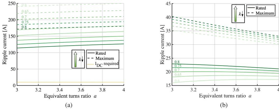
Figure 4.12: The worst leakage ripple current with different coupling factors and effective turns ratios on (a) primary side and (b) secondary side
