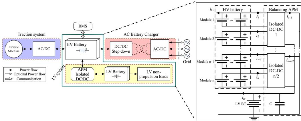
Figure 2.11: Simplified EV system architecture with proposed APM
