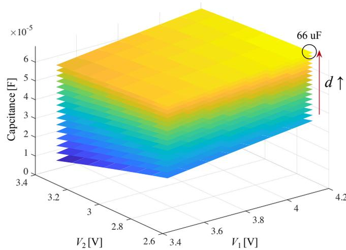
Figure 3.14: Required capacitance with different cell voltages and phase shift
