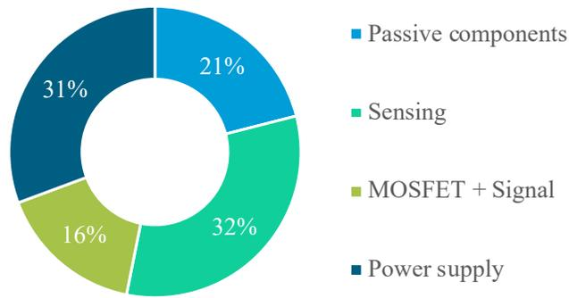
Figure 6.3: The DAHB cost breakdown for optimized batch production
