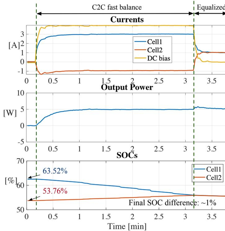
Figure 3.48: Experimental balancing functionality tests on two 3000 mAh NMC cells with 4 A C2C with 5 W load when balancing
