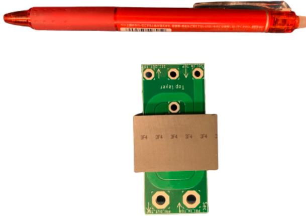
Figure 3.34: The assembled transformer for HFB
