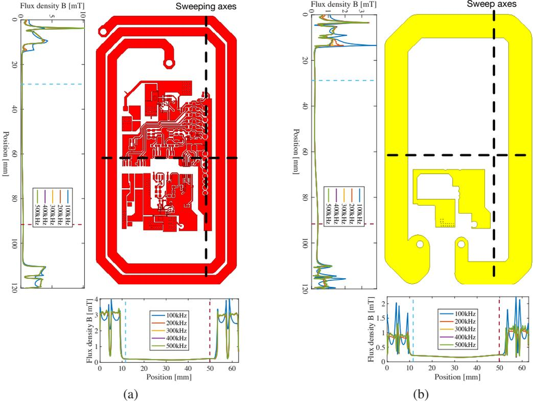
Figure A.1: The flux density distribution on (a) the top and (b) layer-2 PCBs
