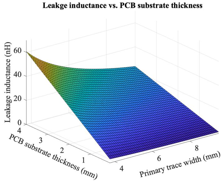
Figure 3.23: The correlation between leakage inductance and other PCB design parameters
