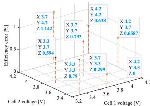
Figure 5.20: The error between ground-true maximum efficiency and MPPA efficiency
