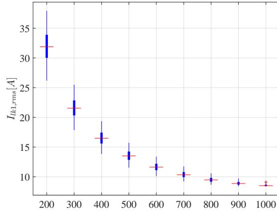
Figure 5.6: The RMS current for a 10 W load at different frequencies
