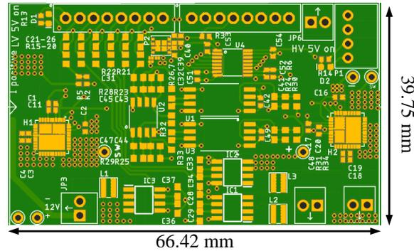
Figure 4.24: The dimensions of the main component board
