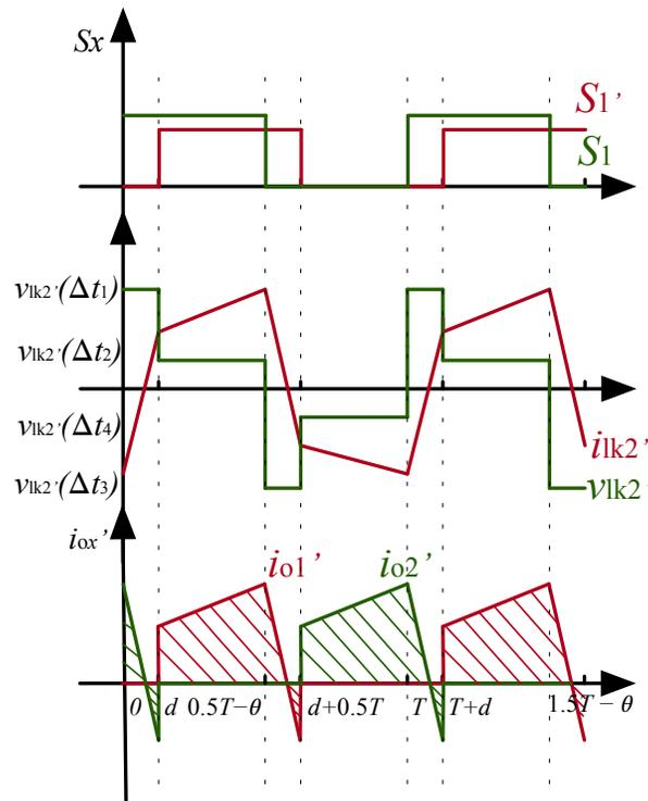
Figure 4.15: The necessary waveforms to calculate the secondary leakage inductor value
