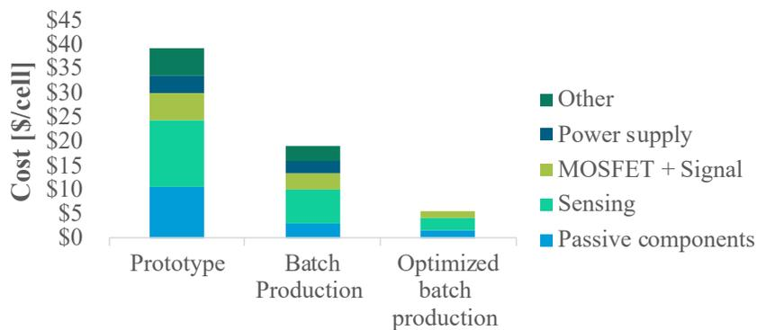
Figure 6.4: The DAHB cost comparison between prototype and batch production in terms of component category
