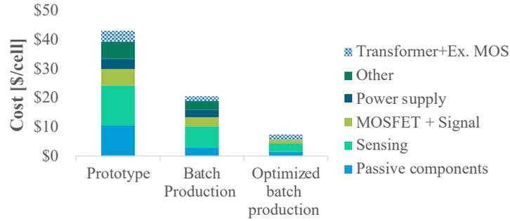
Figure 6.6: The cost comparison between prototype and batch production in terms of component category
