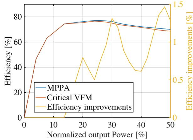
Figure 5.22: The comparison between critical VFM and MPPA-VFM at low load conditions
