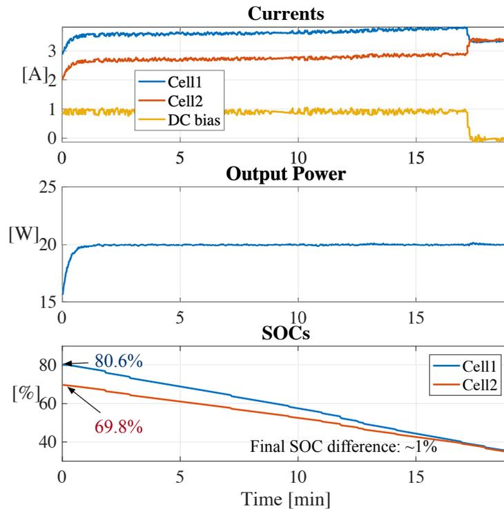
Figure 3.47: Experimental balancing functionality tests on two 3000 mAh NMC cells with 1 A C2C current with 20 W LV load
