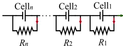
Figure 2.2: The passive balancing strategy - excess energy is dissipated in the paralleled resistors
