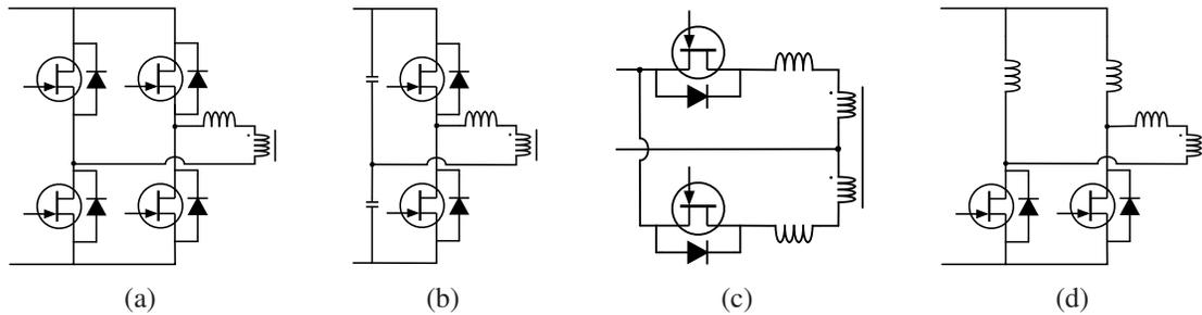
Figure 3.1: Major primary topologies for high-frequency converters: (a) full bridge, (b) half bridge, (c) push-pull, and (d) L-type half bridge
