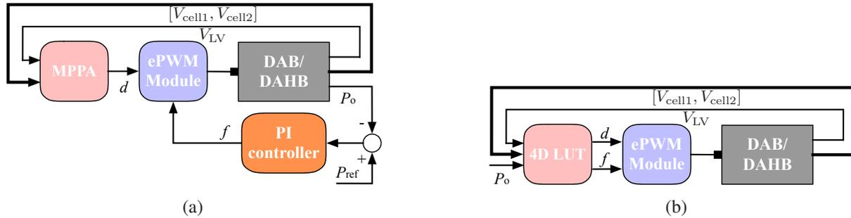
Figure 5.14: The control architecture with (a) direct MPPA-based VFM (b) conventional critical VFM
