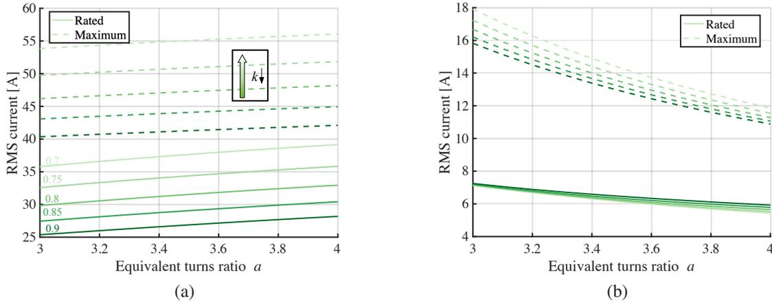
Figure 4.13: The worst leakage RMS current with different coupling factors and effective turns ratios on (a) primary side and (b) secondary side
