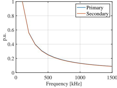
Figure 5.7: The p.u. changes of products  $F_r^{\text{pri}}(f_s)I_{lk1,\text{rms}}^2$  and  $F_r^{\text{sec}}(f_s)I_{lk1,\text{rms}}^2$  as switching frequency increases for the cored transformer designed in Chapter 3
