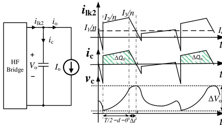
Figure 3.13: Filtering capacitor design, left: equivalent circuit focusing on output, right: output current and voltage waveforms
