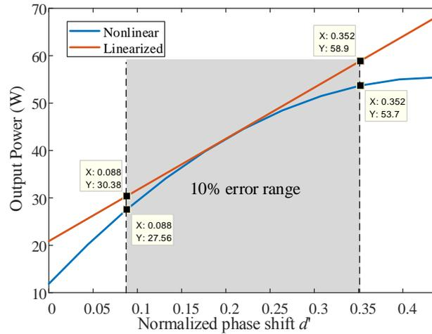
Figure 3.38: Comparison between linearized and original power curves
