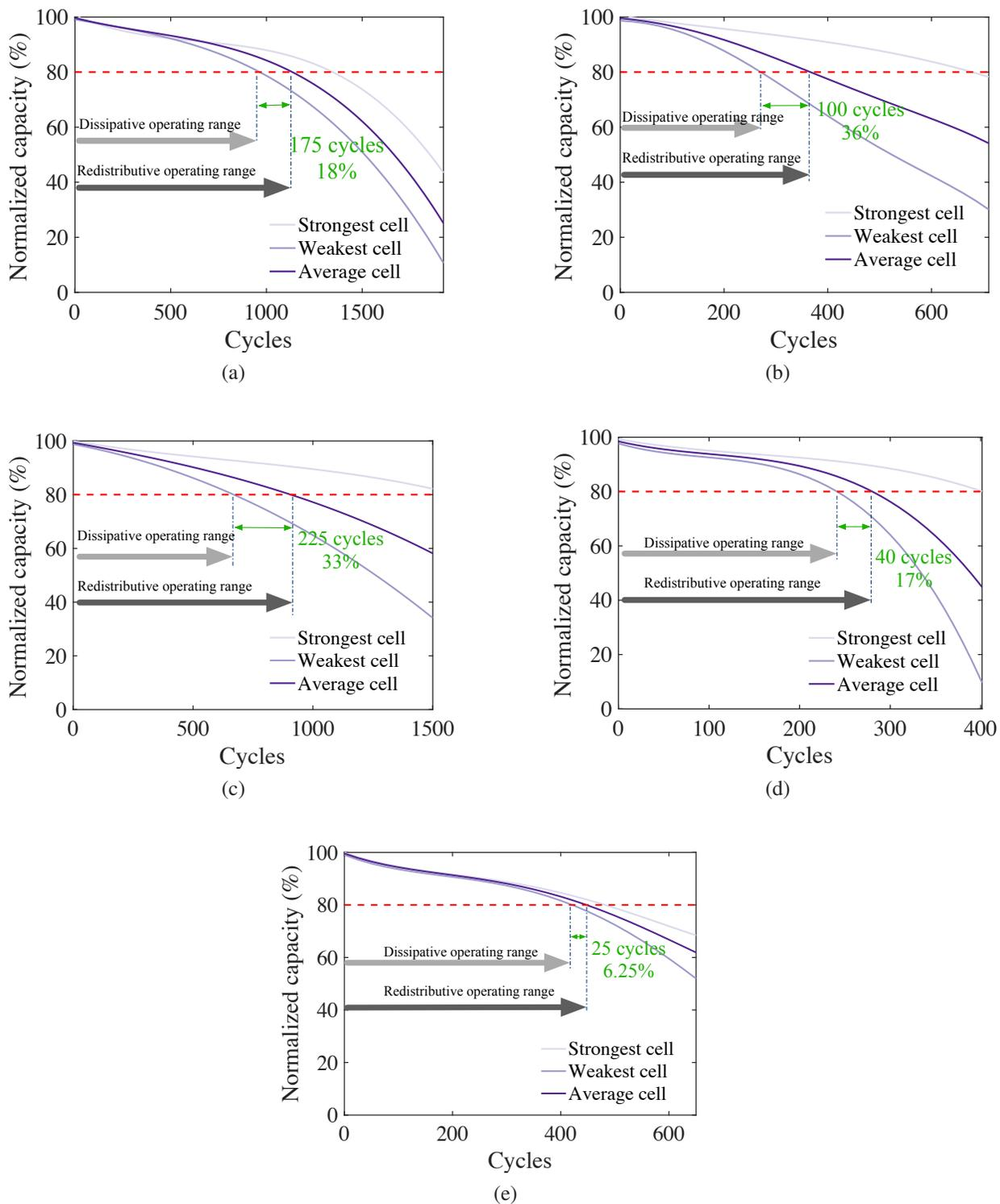
Figure 2.8: Conservative projected life extension of using redistributive balancing in EV application based on cycling data from (a) [29], (b) [30], (c) [31], (d) [32] (e) NMC cycling data
