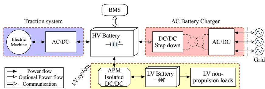
Figure 2.10: The simplified EV architecture
