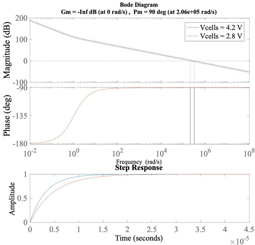
Figure 3.39: The Bode plot for the PI controller of  $\theta$  and its step response
