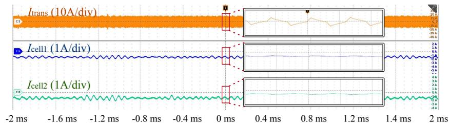
Figure 3.51: Comparison between the measured cell currents and transformer current
