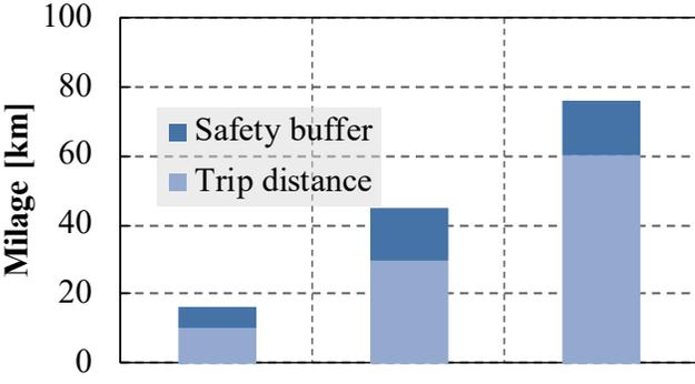
Figure 1.2: The trip distance vs. extra driving buffer due to range anxiety [4]
