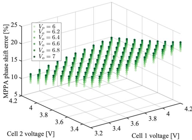
Figure 5.11: The MPPA phase shift error between 1st-order model and full-order one
