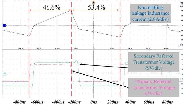
Figure 3.42: Leakage inductor current measurement: asymmetric control regulating unbalanced cells non-drifting
