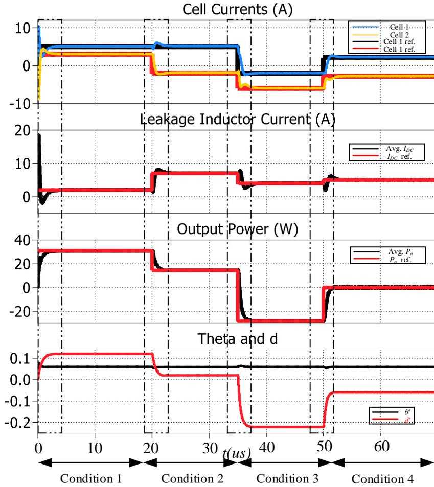
Figure 3.40: Simulated controller reactions to step reference changes
