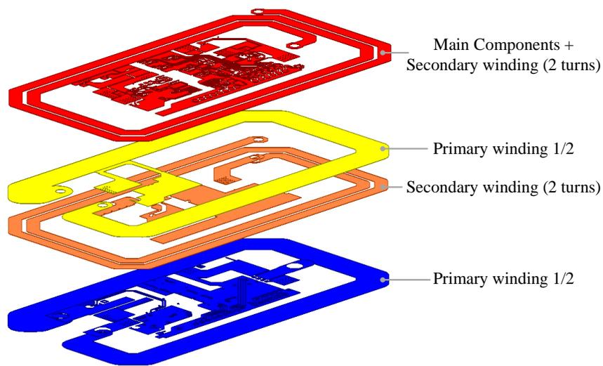
Figure 4.25: The 3D model for FEA in Maxwell/ANSYS
