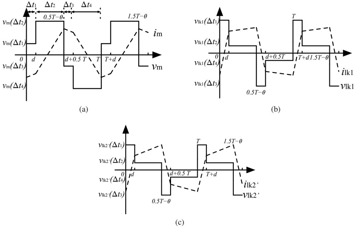
Figure 4.7: The waveforms of (a) magnetizing inductor, (b) primary leakage inductor, (c) primary-referred secondary leakage inductor
