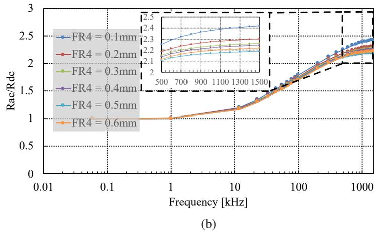
Figure 3.33: The simulated  $F_r$  at different frequency with multiple FR4 thicknesses on (a) primary side and (b) secondary side
