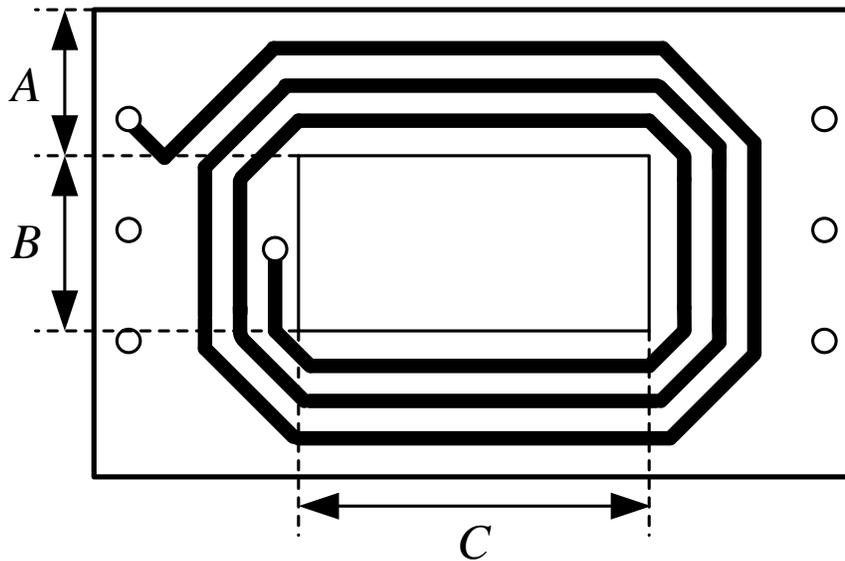
Figure 3.26: The dimensions for calculating the MLT for a rectangular winding
