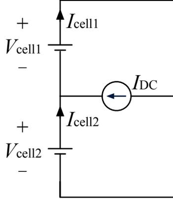
Figure 3.10: The average equivalent circuit model of the primary side
