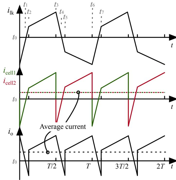
Figure 3.8: The current waveforms when battery are balanced, top: leakage inductor current on primary side; middle: cell currents; bottom: output current on LV side
