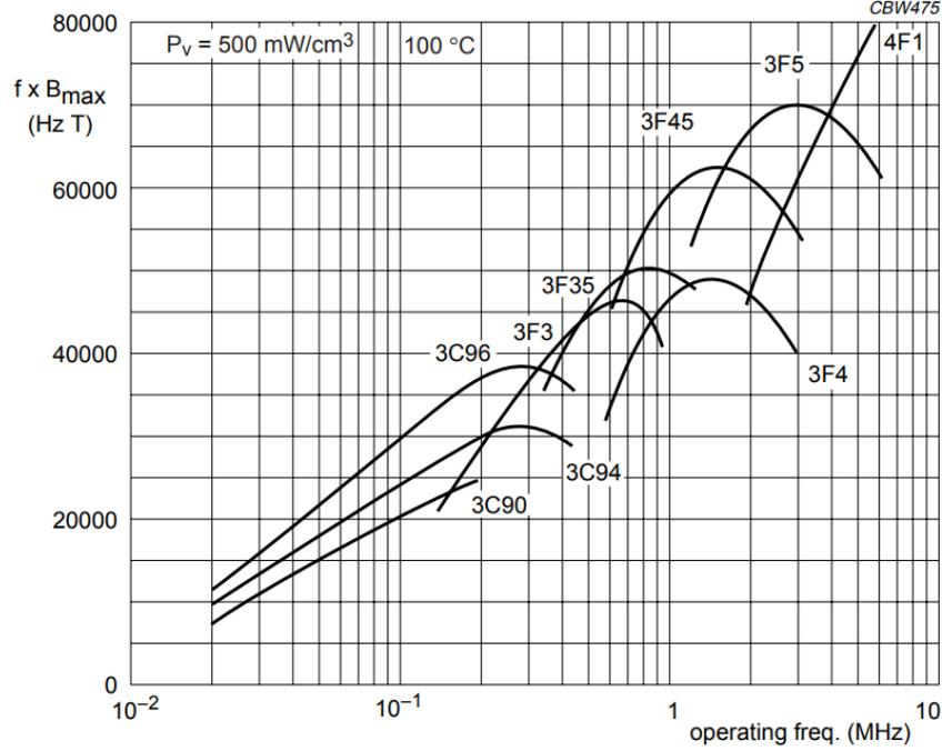
Figure 3.20: The material spectrum used to select core material [64]
