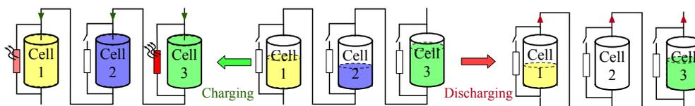
Figure 2.4: The balancing results utilizing dissipative balancing strategy
