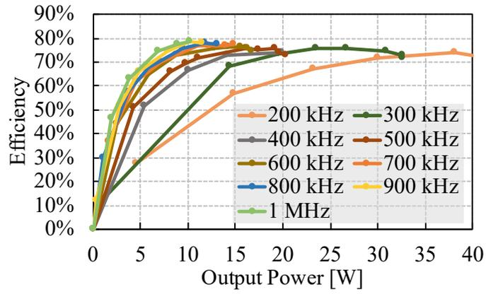
Figure 4.28: The measured efficiency with respect to output power at different operating frequency
