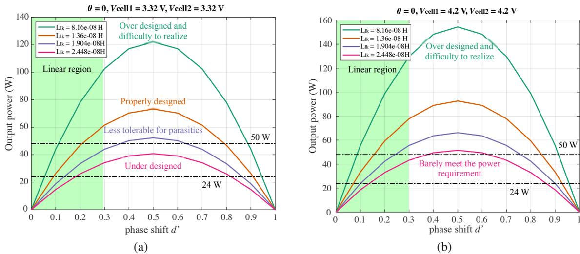
Figure 3.18: The power spectrum with a range of leakage inductance values at 500 kHz when battery cells are (a) at 20% SOC, (b) at 100% SOC
