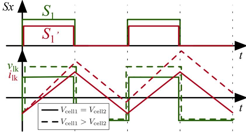
Figure 3.4: The diverged leakage inductor current compared with stable one when cells are unbalanced
