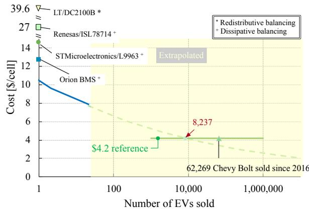
Figure 6.5: The production cost vs. number of EVs sold for the DAHB configuration
