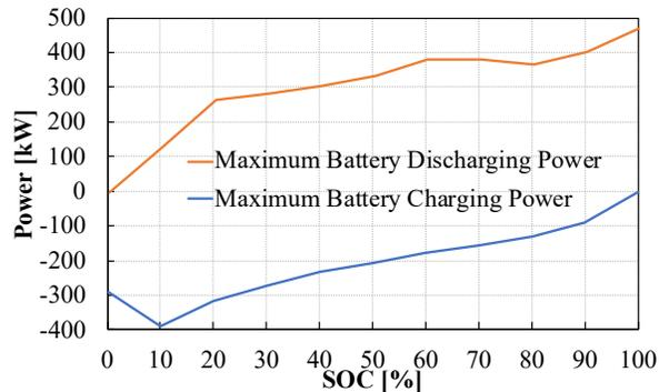
Figure 3.16: Maximum discharging power for Nissan Leaf [62]
