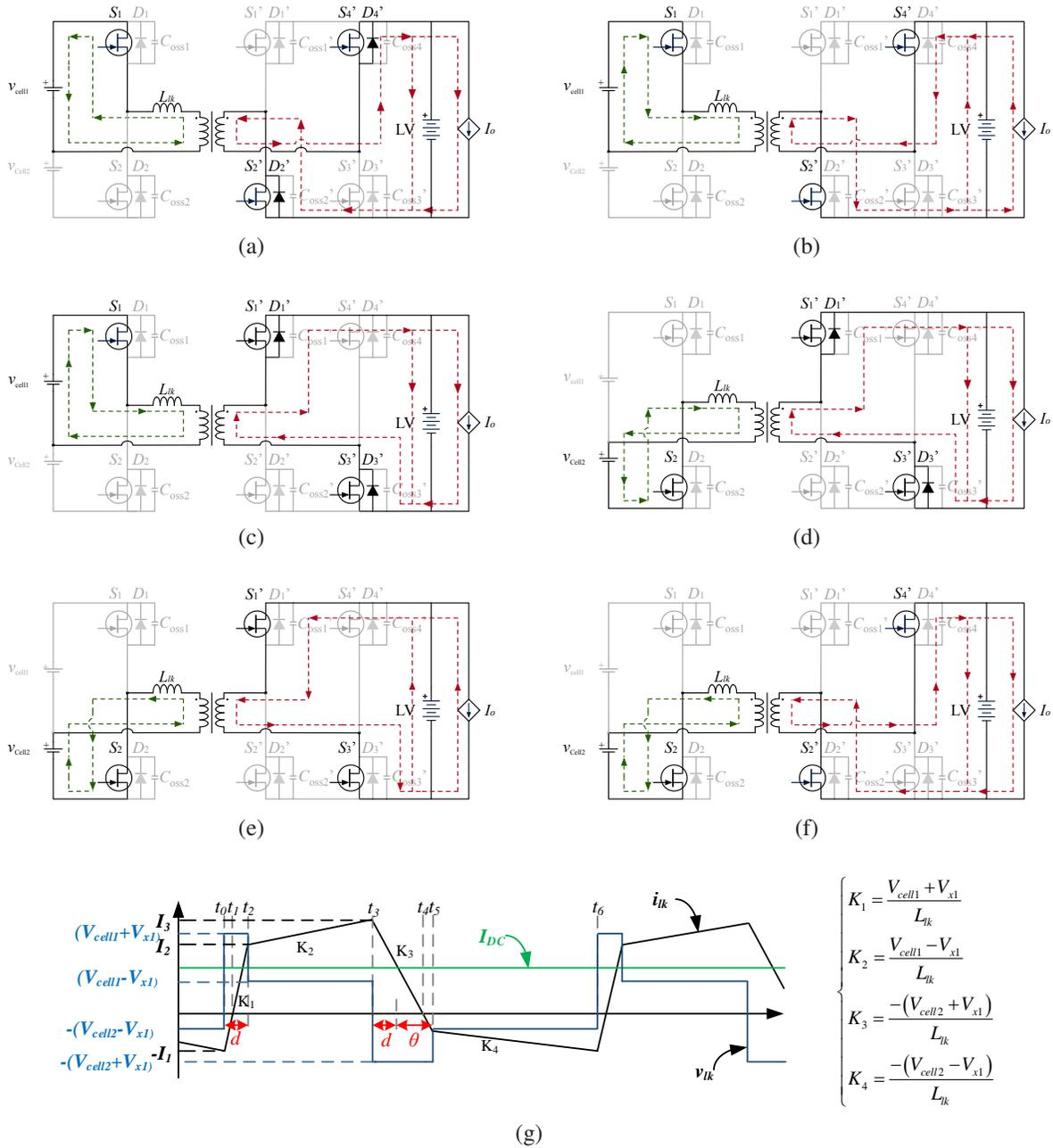
Figure 3.3: Operating states of the HFB, (a) ECM between  $t_0$  and  $t_1$ , (b) ECM between  $t_1$  and  $t_2$ , (c) ECM between  $t_2$  and  $t_3$ , (d) ECM between  $t_3$  and  $t_4$ , 4 (e) ECM between  $t_4$  and  $t_5$ , (f) ECM between  $t_5$  and  $t_6$ , (g) the leakage inductor current waveform with time stamps
