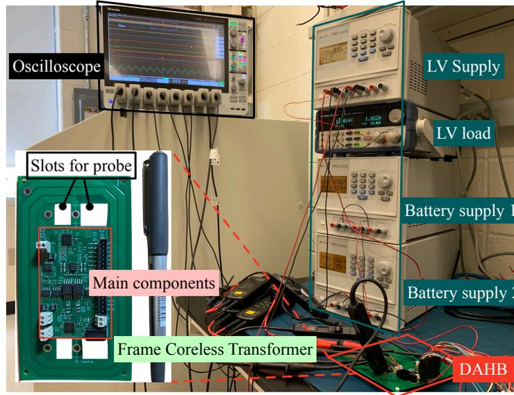
Figure 4.26: The prototype of the proposed DAHB with coreless transformer under testing
