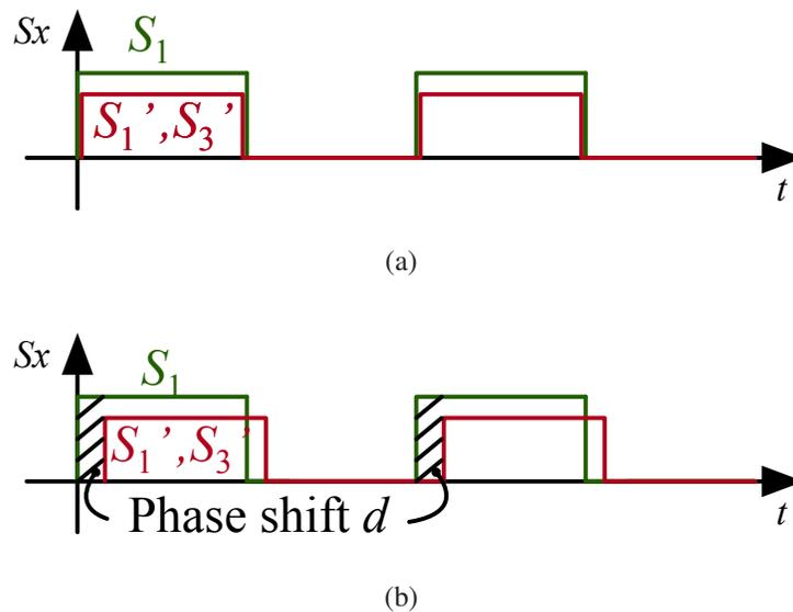
Figure 3.7: The PWM signals (a) without phase shift and (b) with phase shift
