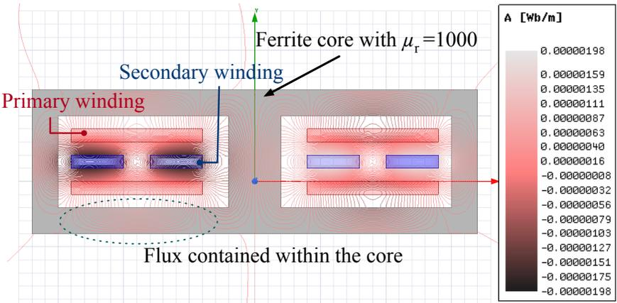
Figure 4.1: Distribution of flux lines for a transformer with core
