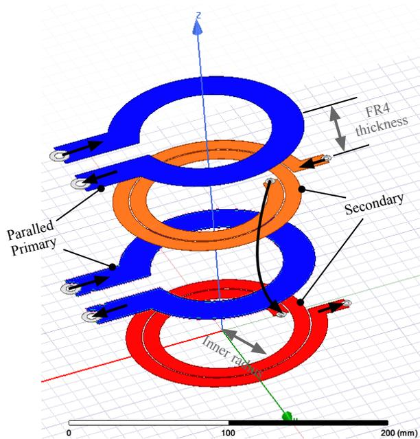
Figure 4.19: The ANSYS/Maxwell model of a helical 4-layer coreless transformer
