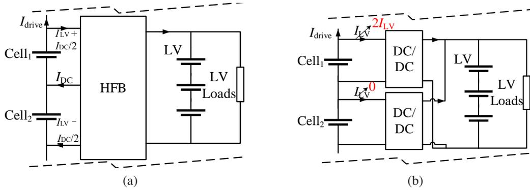
Figure 3.52: Equivalent circuits for simulation using driving cycles: (a) proposed topology, (b) existing topology
