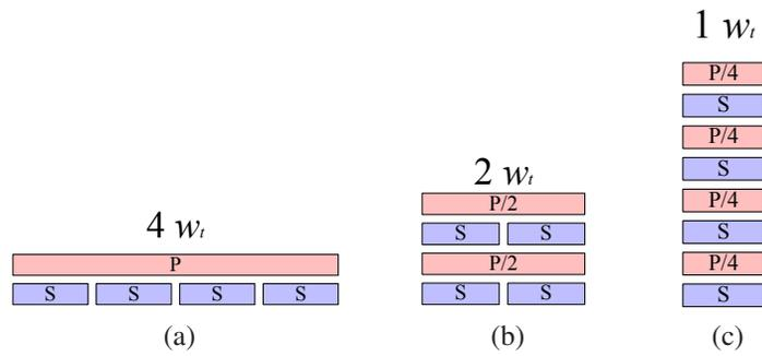
Figure 4.18: The possible planar winding layouts with (a) 2-layer, (b) 4-layer and (c) 8-layer structures (cross-section on one side of the windings)
