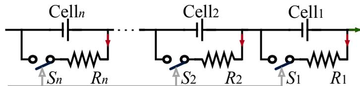
Figure 2.3: The dissipative balancing strategy - excess energy is dissipated in the paralleled resistors by active control
