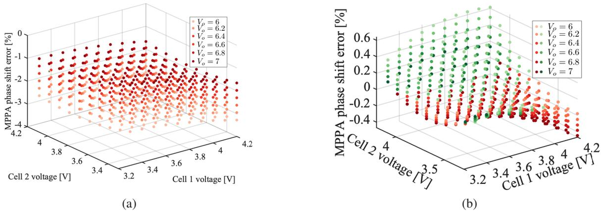
Figure 5.12: The MPPA phase shift error between 2nd-order model and full-order one expanded at (a)  $d = 0.25$  and (b)  $d = 0.35$
