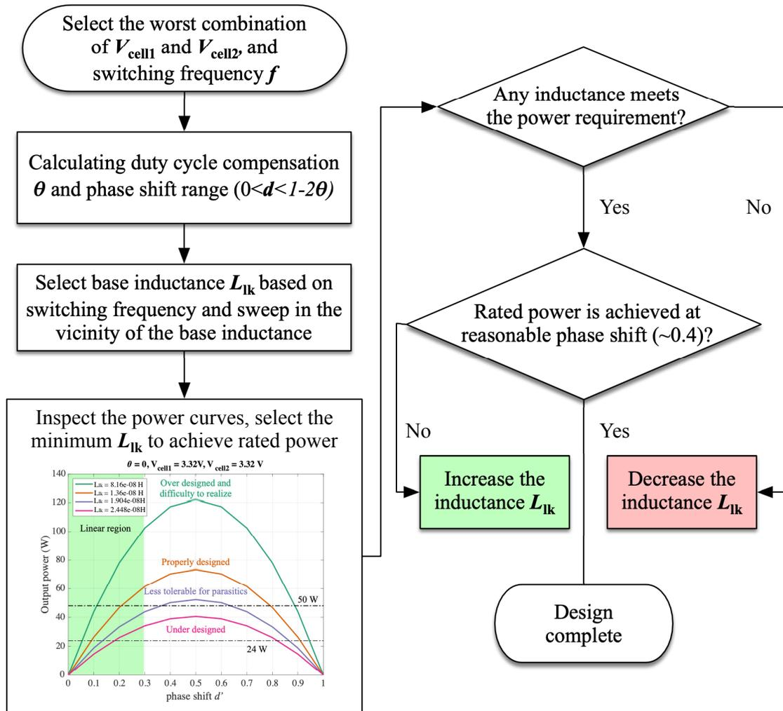
Figure 3.19: Flowchart of selecting leakage inductance to achieve rated power and peak current limitation
