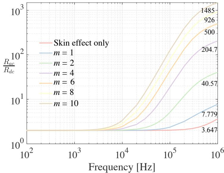
Figure 3.27: The distribution of  $F_r$  across a wide range of frequencies and different number of layers
