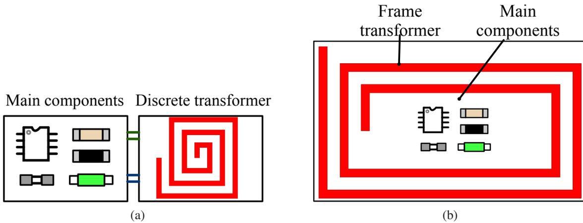
Figure 4.23: The possible transformer layout structures: (a) discrete transformer structure and (b) frame transformer structure
