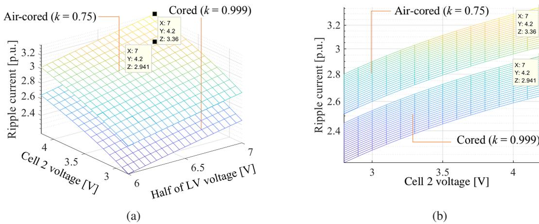
Figure 4.9: Per-unit magnetizing inductor ripple current with the same total inductance: (a) 3D view (b) side view
