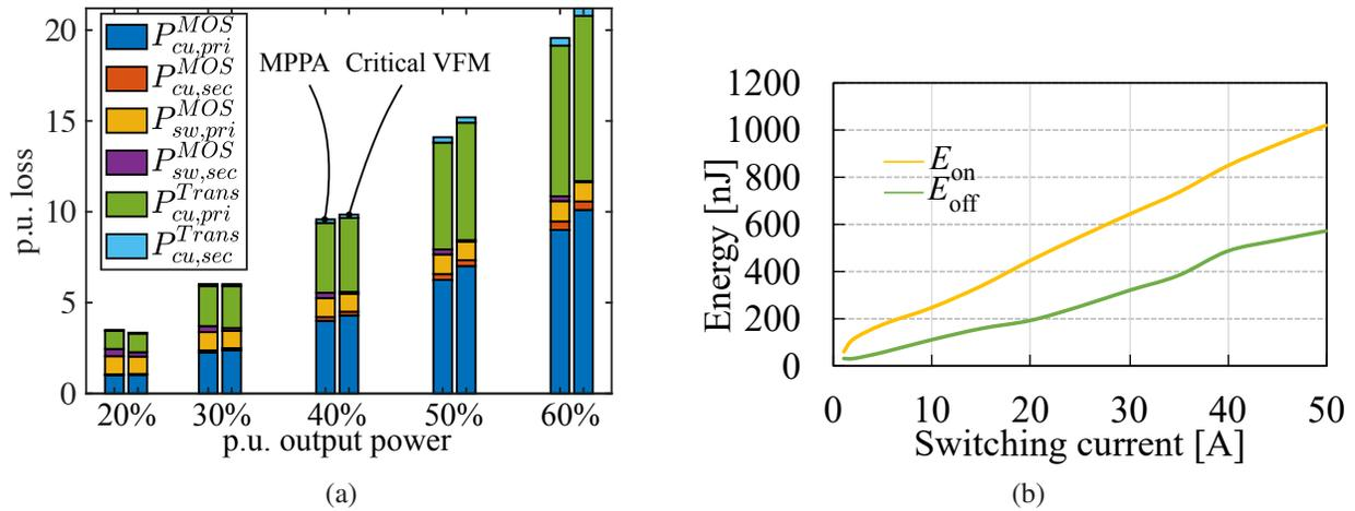
Figure 5.19: (a) The example p.u. loss distribution between MPPA-VFM and critical VFM at different power levels; (b) The extracted switching energy from double pulse test using the SPICE model
