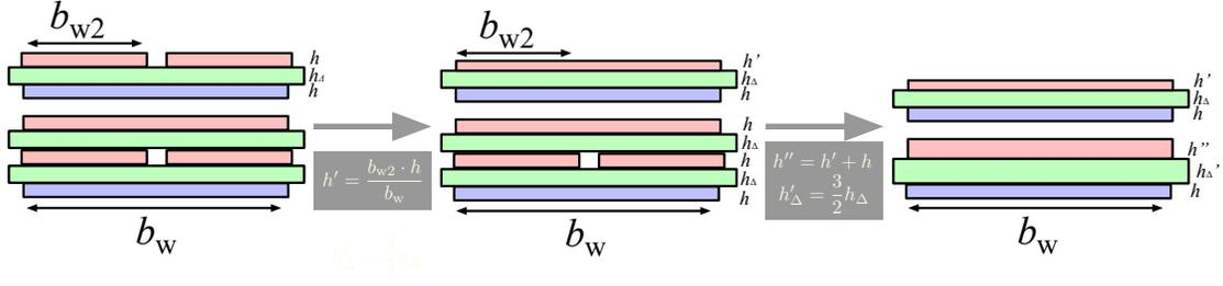
Figure 3.30: The steps to convert asymmetrical fully-interleaved structure to symmetrical fully-interleaved one
