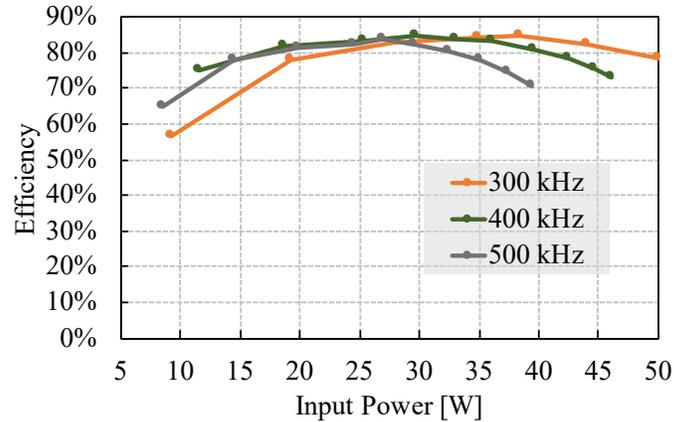
Figure 3.50: The efficiency measurements of the proposed HFB
