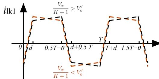
Figure 4.8: The waveforms of the primary leakage inductor current when Eq. (4.18) is satisfied and unsatisfied
