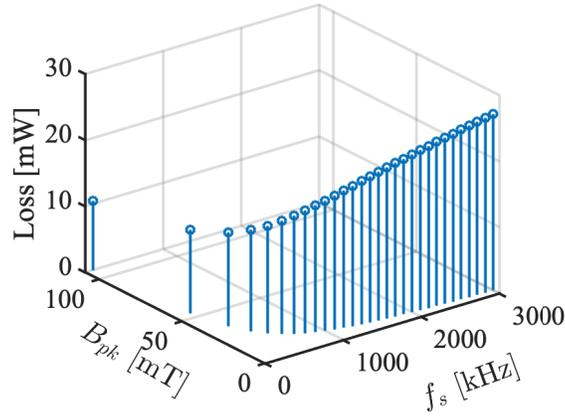
Figure 5.8: The core loss varying with frequency
