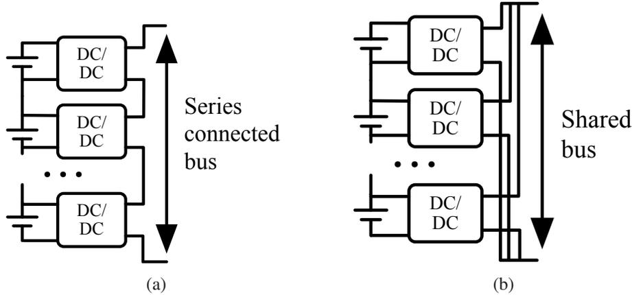
Figure 2.7: Converter-based battery balancing structure: (a) series modular design, (b) parallel modular design
