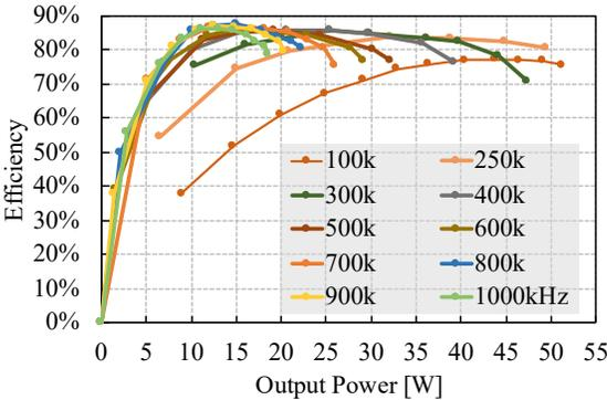
Figure B.2: The measured efficiency of the HFB system with coreless transformer
