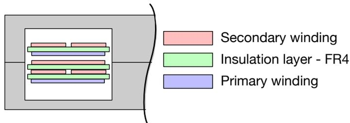
Figure 3.24: Winding layout
