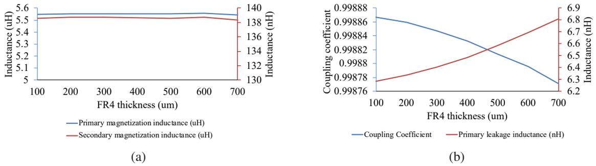
Figure 3.32: The correlation between FR4 and (a) magnetization inductances, and (b) leakage inductance
