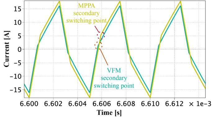
Figure 5.18: The waveform comparison between MPPA and VFM at 200 kHz
