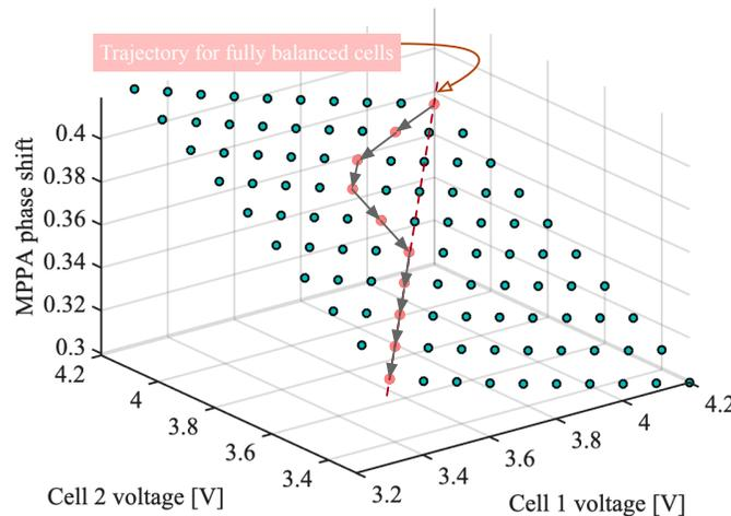
Figure 5.15: The example trajectory of MPPA phase shift as the cells discharge from full
