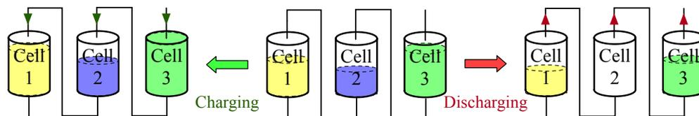
Figure 2.1: The consequences of charging or discharging unbalanced battery cells in series connected configuration
