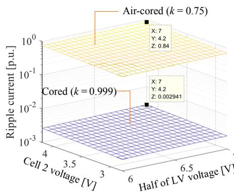
Figure 4.10: Per-unit magnetizing inductor ripple current with the same leakage inductance in log scale
