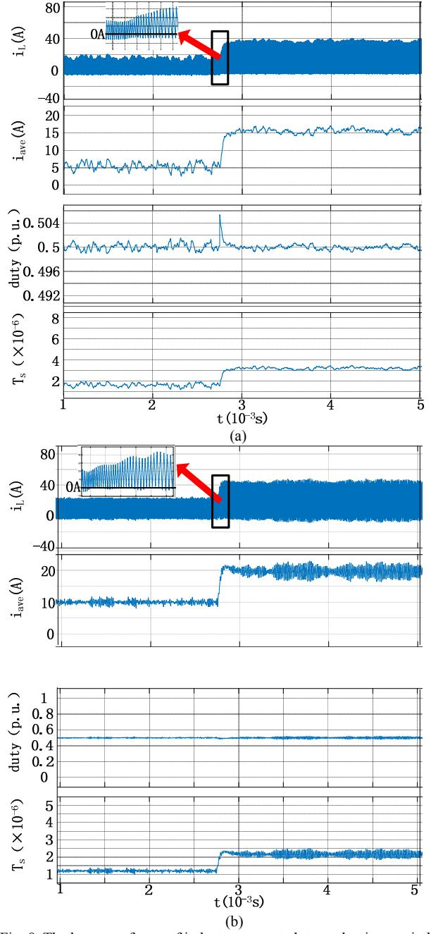
Fig. 8. The key waveforms of inductor current, duty cycle, time period between (a) proposed MPC method and (b) PI.
