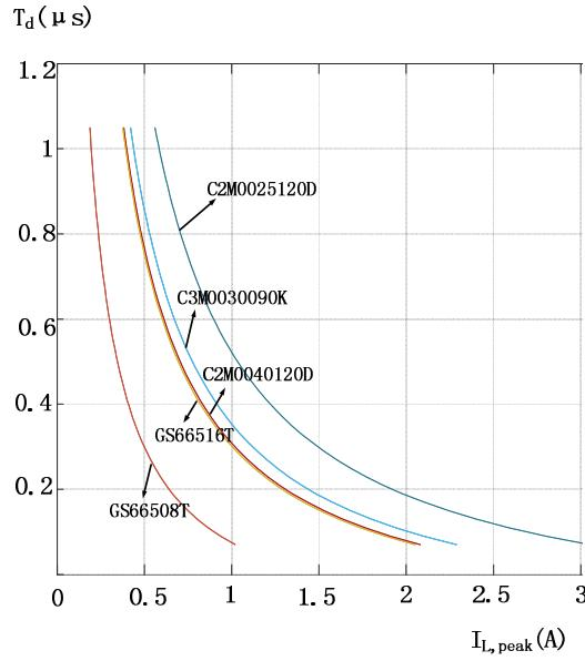
Fig. 5. The soft switching operation regions for different devices.
