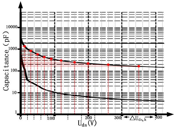
Fig. 3. The discrete points of output capacitance with  $U_{ds}$ .
