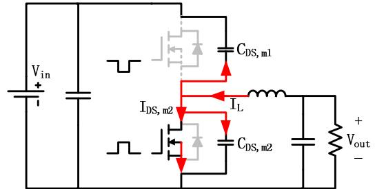
Fig. 1. The negative inductor current paths.
