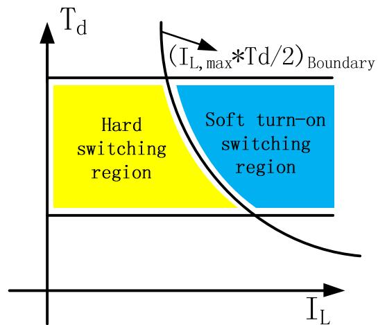
Fig. 4. The boundary conditions for critical soft switching.
