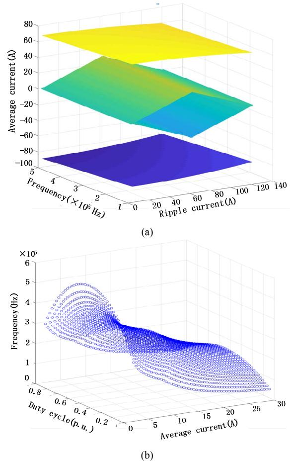
Fig. 8. The thermal, soft switching, frequency and device current constraints (a) of  $\Delta i_L$  with the function of  $f_{sw}$  and  $I_{ave}$  (b) the optimal  $f_{sw}$  regions with relationship of duty and  $I_{ave}$ .
