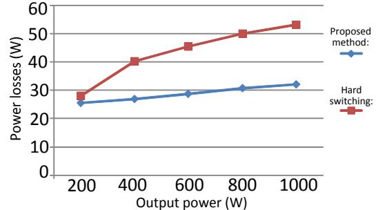
Fig. 10. Power losses comparison between proposed method and hard switching.
