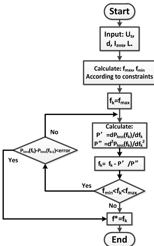
Fig. 7. The power losses optimization flow chart.
